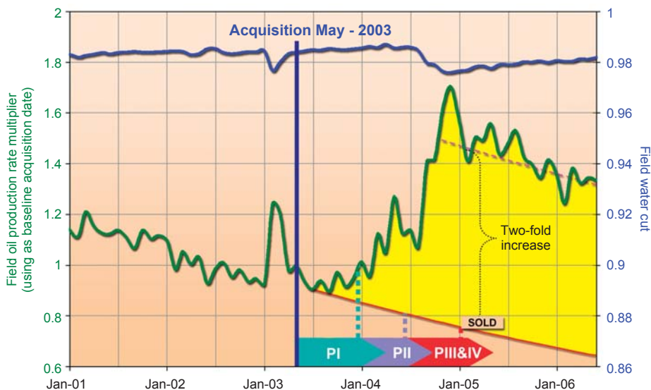
Fieldwide Oil and Water Production (Before and After Applying the Four-Phase Methodology)
